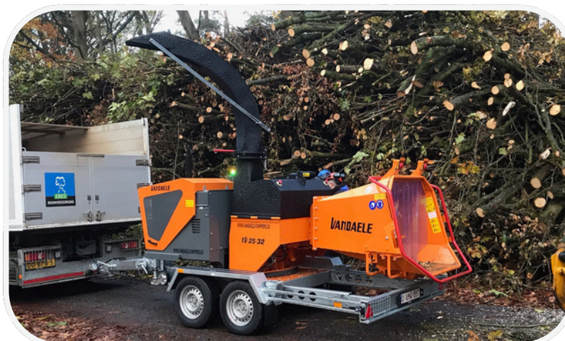
Machine version rotatable on a chassis with double-wheel axle and a height-adjustable drawbar. Available in a tracked version with a rotating upper structure.
