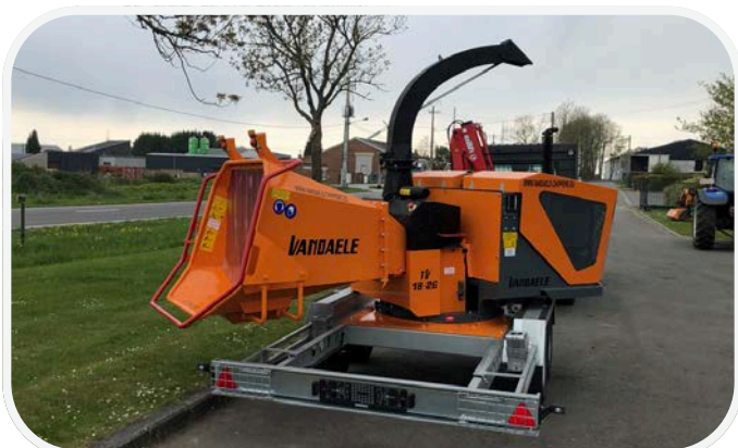
Machine version rotatable on chassis with double-wheel axle and height-adjustable drawbar
