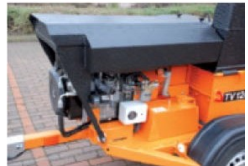
TVI 20 D; Air cooled LOMBARDINI diesel engine, 2 cylinder, 21 kW - 28.5 HP.
