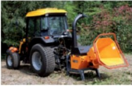
TVI 20 P; Can be powered by small tractors, as from 20 HP.
