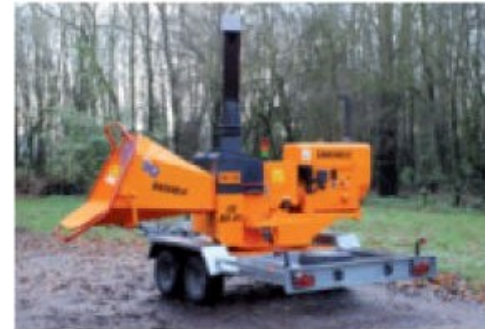
TV20-26 D ; Diesel engine version, standard mounted on a 360° turn able double axle trailer;
