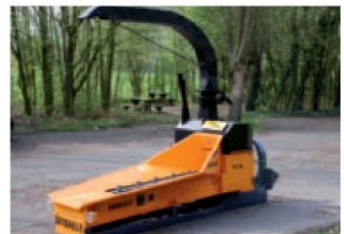
Option crane funnel – version with extra long feed table and chain.
